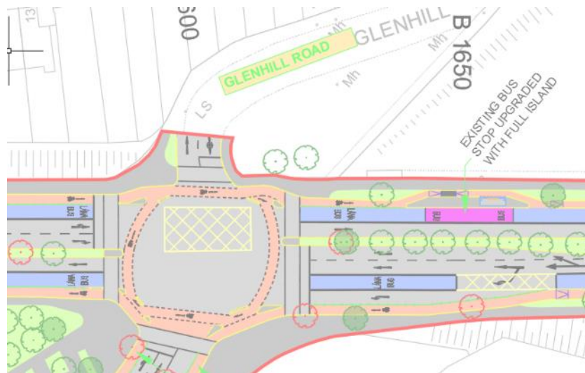
Figure 2-2 Junction Type 2 Proposed Glenhill Road Junction
